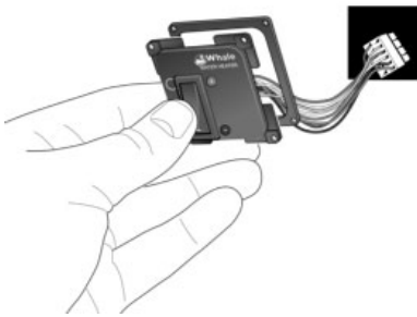
Fig. 17 Insert control panel
