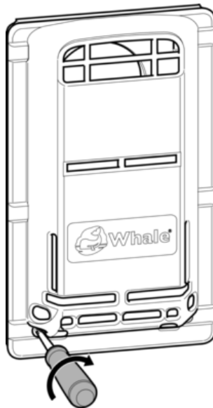
Fig. 11 Installation and securing of flue cover
